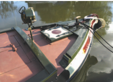
below left Good access but no weed hatch for the bow thruster.
